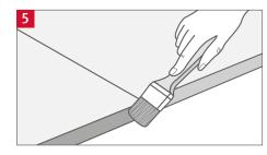
Seal any exposed mechanical fixings, perimeter edges, cut edges and stairwells using EGGER Joint & Joist Adhesive. Once the building is watertight, excess adhesive can be removed with a scraper.
