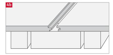
All short end joints should always fall on the centre of a secured joist, including perimeter edges. Where this is not the case, please refer to the relevant building guidelines.
