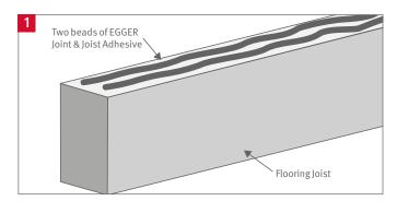
Apply two parallel beads of EGGER Joint & Joist Adhesive to the top of the joist along the first row of boards.
