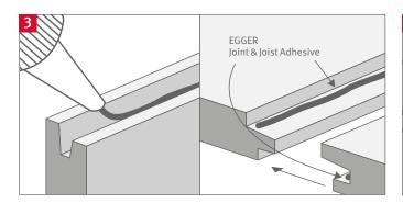
Apply EGGER Joint & Joist Adhesive directly to the groove and shoulder of the profile joint, continuing down the length of each board to ensure that the entire joint is bonded once the boards are butted tightly together. Adhesive should foam out of the board joint. This will enhance the protection of the joint. Excess adhesive should be left to dry.
