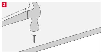
Lay the boards across the joist and fix the first row of boards with only one mechanical fixing (2.5 times the board thickness) per joist along the perimeter edge, minimum 8 mm from the joint edge.
