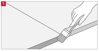
Exposed fitting heads, perimeter edges, cut edges and stairwells must be sealed using EGGER Joint & Joist Adhesive.
